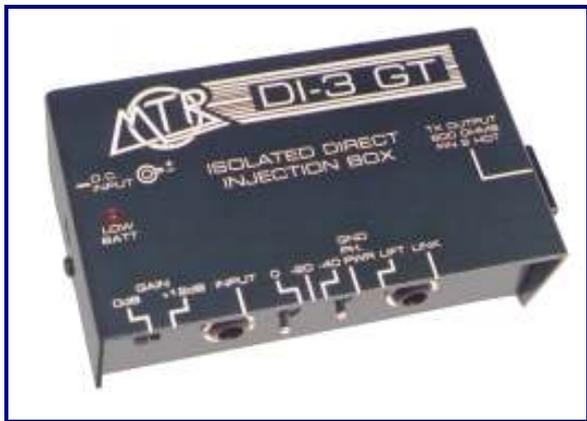
Or thirdly, if the console has phantom power, this can be used just by connecting the output XLR to the mixer's input, up to a maximum of 48 volts. The DI-3GT will reduce this to the required 9 volts. The battery can be left in place, but if a battery is not fitted we suggest that the plastic sleeve supplied is left over the end of the battery cable clip to prevent possible shorting.
