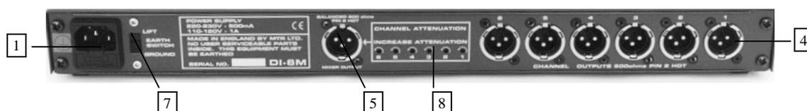
To use the mixer function, insert the screwdriver supplied firmly into the rear panel holes (8) and locate the flat edge into the slot of each trim pot. Turn to adjust each output between zero (fully left) and maximum. This combined signal appears at the Mixer Output socket.
