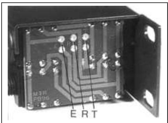
To convert to 'un-normalised' use, scratch hard with a sharp point through the silver-coloured track marked "T" (tip) on the printed circuit board, to make a clean break through the track. Also cut the track marked "R" (ring) if using balanced connections. These breaks can be re-soldered at a later date if your requirements change. Un-normalised pairs are usually used for frequently changing patches such as auxiliary sends and returns, etc.
