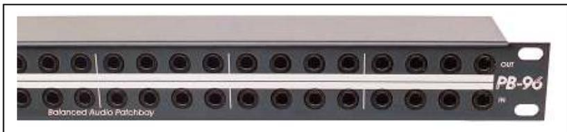
The unit is supplied from the factory 'half normalised', i.e. when nothing is plugged into the front, the top rear jack is connected to the bottom one of a pair, until a jack plug is inserted into the bottom front socket. When this happens, the link
